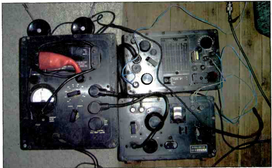
Shown here is the venerable GRC-109 "spy set" used by the CIA and the U.S. Special Forces (Green Berets) from the 1950s into the 1980s. The three boxes shown here comprise the basic radio set. This set can be powered from various sources of AC, 6 VDC, and a hand-cranked generator. The complete radio set weighs in at over 50 pounds and would be a real treat to jump with into a hostile drop zone.
