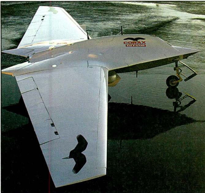
British Corax UAV prototype (not yet wearing stealth material coatings) resembles the Lockheed Darkstar. (Photo courtesy BAE Systems)
