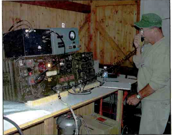
Both of these shots show Ted Young, W3PWW, of Hanover, Pennsylvania, running the Old Military Radio Net using his GRC-19 set. This radio set consists of a T-195 200-watt transmitter, running AM/SSB/CW or RTTY, and an R-392 receiver. This HF set is massive and was the mainstay of battlefield comm gear from the 1950s through the 1980s. The transmitter has a very "innovative" electro-mechanical auto-tune antenna matching unit. It makes a lotta noise, and it is really cool!
