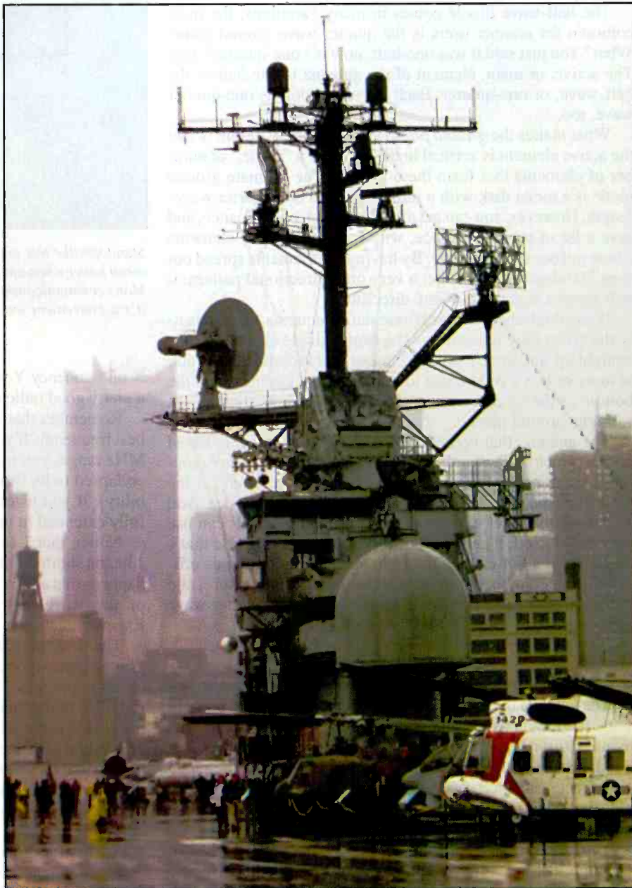
Getting the antenna high and out of the way is more than a function of distance for this impressive array of ship antennas. The salt water sea makes a great ground plane, but the ship itself would shield just about anything that tried to get out if it wasn't high and outside the main structure.
