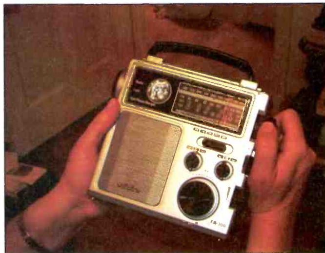
The tuning dial is analog with a co-located coarse and fine-tuning knob.
