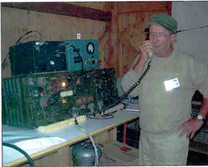
Both of these shots show Ted Young, W3PWW, of Hanover, Pennsylvania, running the Old Military Radio Net using his GRC-19 set. This radio set consists of a T-195 200-watt transmitter, running AM/SSB/CW or RTTY, and an R-392 receiver. This HF set is massive and was the mainstay of battlefield comm gear from the 1950s through the 1980s. The transmitter has a very "innovative" electro-mechanical auto-tune antenna matching unit. It makes a lotta noise, and it is really cool!
