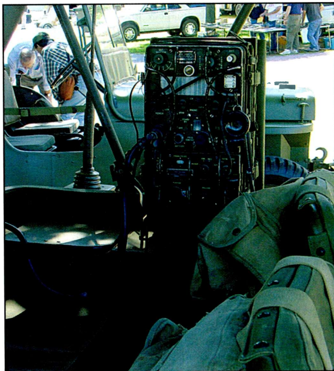
This is one place you can find a GRC-9—the back of a “flat-fendered” jeep. Notice the T-18 mic. The GRC-9 is a great piece of MilCom gear for CW and AM phone work. It’s “cute” in a weird sorta way.
