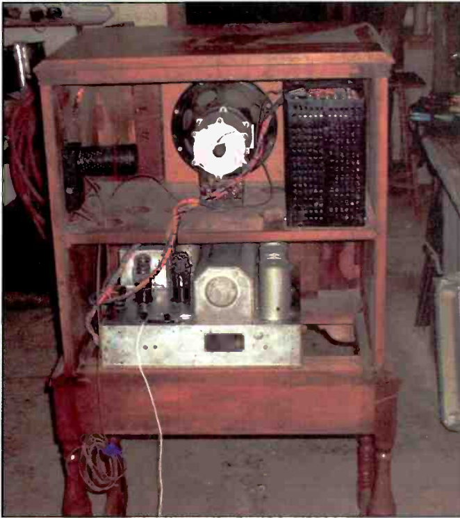
Photo B. Here's how it all goes together! The speaker, chassis, power supply, and ballast tube assembly can be seen in the rear view of the cabinet. The set should have a ventilated rear cover to prevent contact with the exposed high voltages and hot surfaces on the ballast and tube surfaces.
